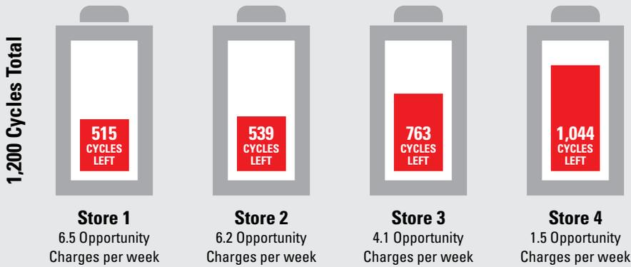
To get a sense of how the NexSys® batteries have fared fleetwide so far, consider the battery cycling data highlighted in the chart – these four locations represent some of the lightest and heaviest usage of the 33 NexSys battery installations.
